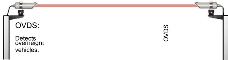
Dual Single Eye OVDS installed outside parking structure detecting two different heights.
