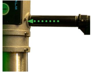
3. Thread the supplied mounting feet onto the other three support elbows. Using a large bolt and gasket removed in step 1, affix the support elbows to the bottom of one beacon housing, and to the top and bottom of the other housing. Use the supplied self tapping screws or banding to affix the lower beacon to the pole.
