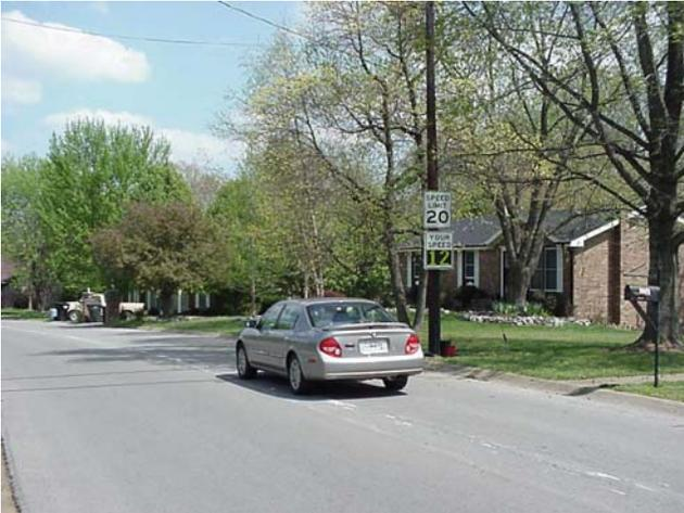
All three field studies showed positive speed reduction results. In each study, speed was measured before the deployment of Driver Feedback Signs and at various times after the deployment. All were permanently mounted signs.
