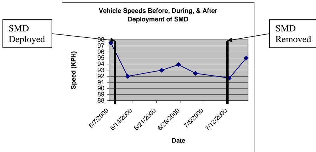
Portable speed monitoring displays are useful in situations where temporary speed reductions are necessary, such as work zones. Areas with recurring speed management needs such as schools zones, residential areas, and speed transition zones require a permanently mounted solution.
